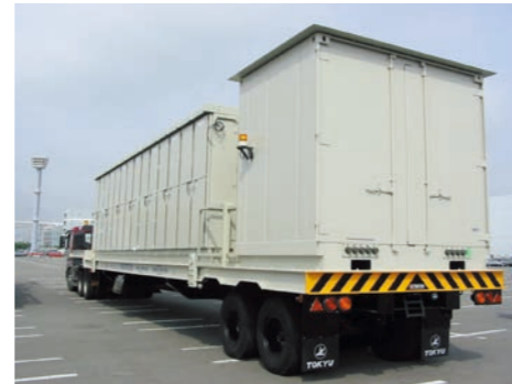
Right : Trailer B, MV Switchgear & LV Control-gear
